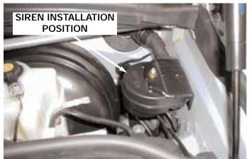
The rechargeable battery will allow the siren to sound if it or the vehicle's battery is dis-connected. The siren battery is recharged, from the vehicle's battery when DWA is not in the armed state.
